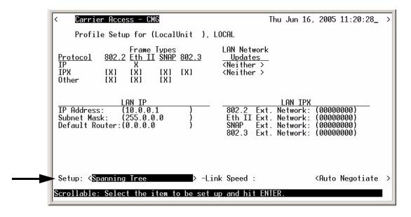
4. To enable Spanning Tree, scroll **<Disabled>** to **<Enabled>**, with the **[SPACEBAR]**, select **[ENTER]**.
